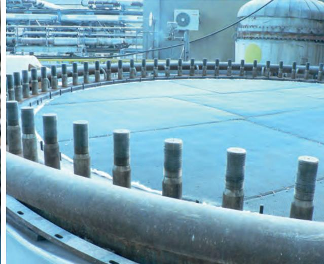
A multistage catalyst from Heraeus is installed in a fertilizer plant; source: Heraeus
