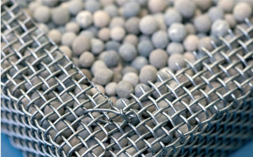
Anti-nitrous oxide granulate: Small spheres encased in precious metals destroy nitrous oxide produced in reactors for manufacturing nitric acid.
