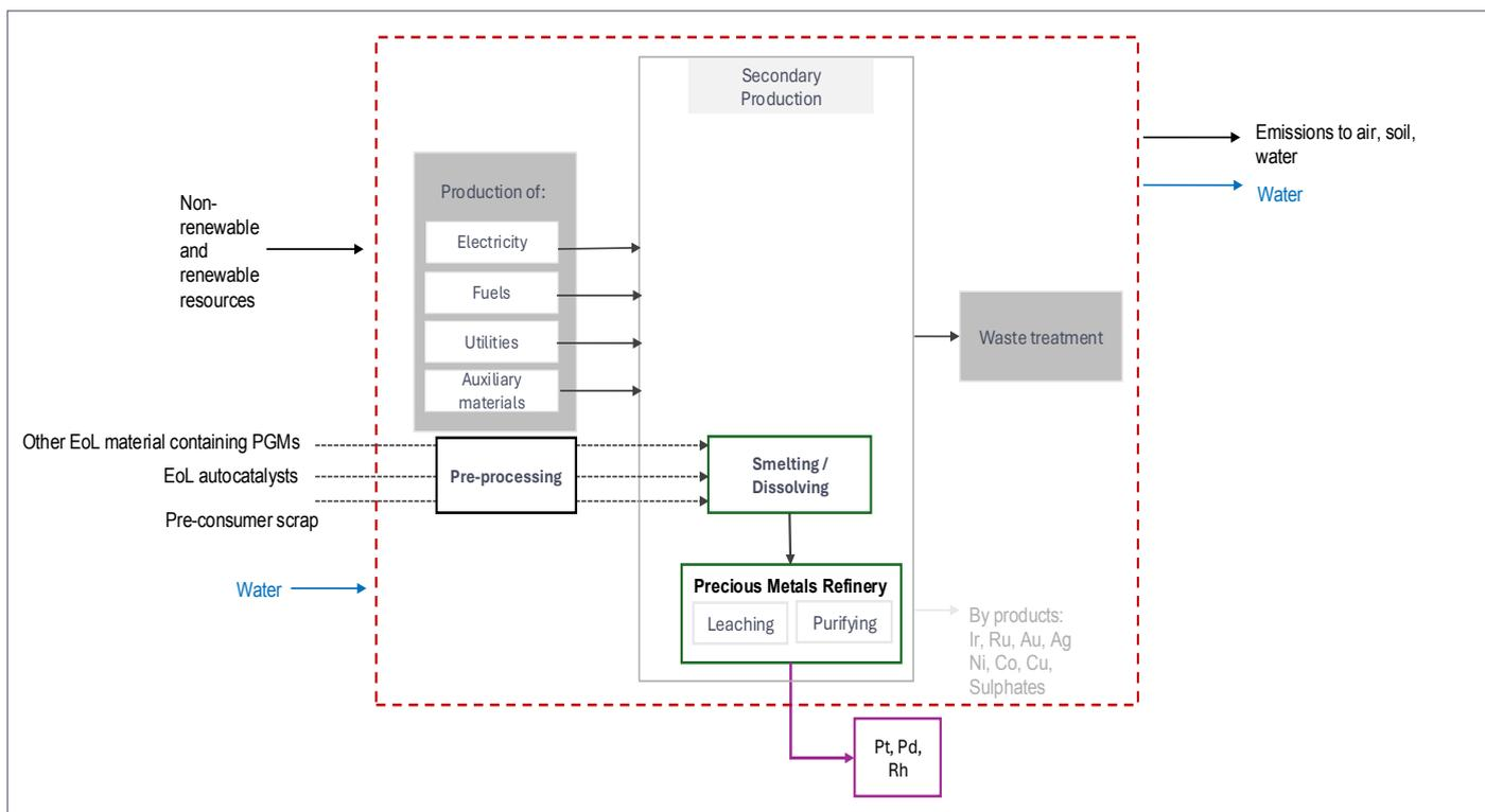
Figure 2: System boundary for secondary production
