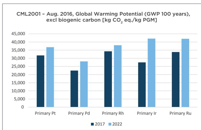
Figure 8: GWP comparison for primary production of 1 kg PGM between 2017 and 2022 production data
